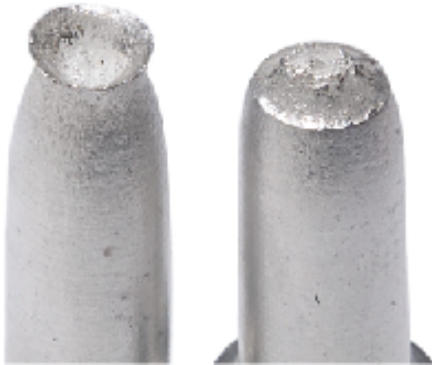
cup-and-cone fracture in aluminum
