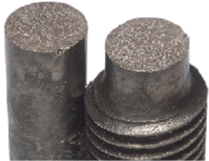
brittle fracture in a mild steel
