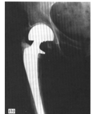
Hip implant-cyclic loading from walking.
